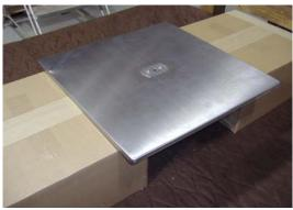
**2-** To protect the stainless surface against scratches, the protective film can be left on the base plate until the assembly is complete. If the base plate did not come with the protective film, strips of masking tape can be placed over the alignment washer to protect the stainless surfaces against scratches. **Note**: The masking tape is not necessary if caution is taken to not scratch the stainless surface.
