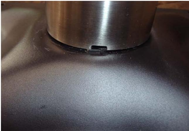
**6-** Inspect to see that all of the tabs are securely in their slots. Use the supplied tool to firmly tighten the nut. If the tabs did not initially slip into the slots, lightly tighten the nut enough allow some movement, so the tabs and the slots can be properly lined up. When they are aligned, tighten the nut some more and lightly jiggle the column or the mounting plate. The tabs should pop in the slots. Now tighten firmly.
