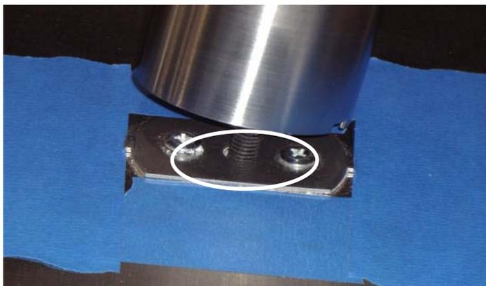
**4-** Put the end of the long threaded bolt into the hole of the alignment washer. Once this is done, align the 2 tabs of the alignment washer with the 2 slots in the column.
