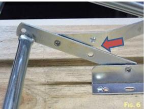
6. As you continue lifting the leg, the pivoting arm will move forward and lock itself into place on the convex divot in the opposing direction. The horizontal cross-bar will prevent it from over extending. Some pressure may need to be applied to ensure it is locked into place (see Fig. 7).
