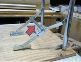
\*Be sure to notice that the horizontal cross-bar is located above the pivoting arm after lifting the leg to the upright position (see Fig. 8). If the cross-bar is below the pivot, it is backwards and will not lock properly. This means the legs will need to be disconnected from the table. Bend the arm in the opposite direction and then reconnect it to the table top in the correct position.
