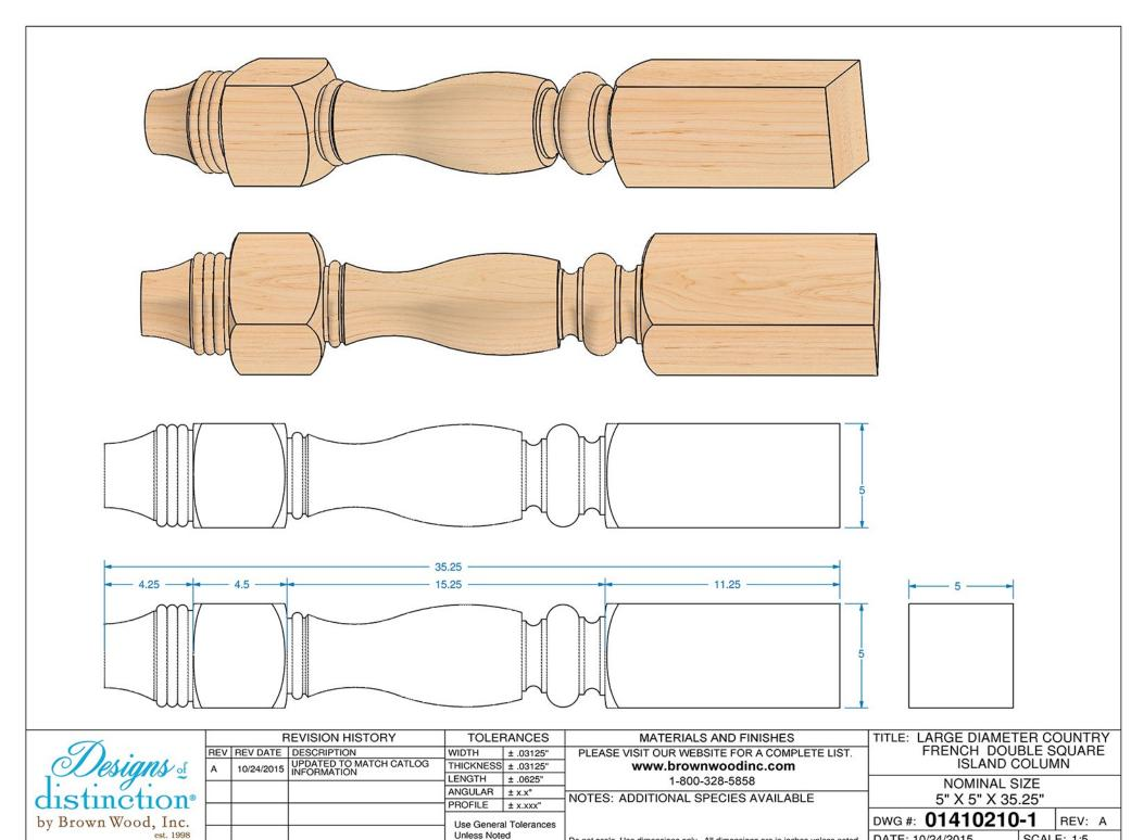
est. 1998 Unless Noted Do not scale. Use dimensions only. All dimensions are in inches unless noted DATE: 10/24/2015 SCALE: 1:5
