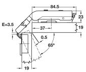
19 mm door thickness Mounting plate height 0 mm
