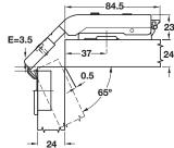
24 mm door thickness Mounting plate height 0 mm
