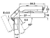
16 mm door thickness Mounting plate height 0 mm
