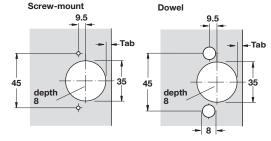
Material: Cup: Zinc, die-cast; Hinge arm: Steel; Finish: nickel-plated
