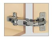
At opening angle of  $90^{\circ}$  and mounting plate height = 0 mm, the door swings out laterally 2 mm when opened.
