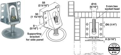
Requires a Ø15 mm hole in the cabinet bottom for adjustment.
