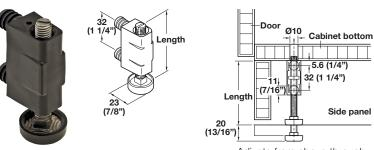
Adjusts from above through a hole in cabinet bottom and from below with an open-ended wrench.
