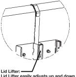
Lid Lifter easily adjusts up and down to provide a greater degree of flexibility when raising the TV out of the cabinet
