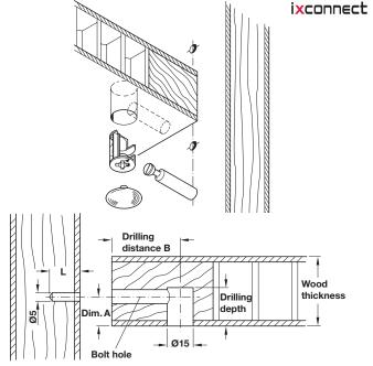
Drilling distance B: Distance from center of Minifix housing to front edge 24 or 34 mm, depending on choice of connecting bolt
