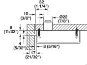
For door thickness: 13–26 mm (1/2"–1") Minimum cabinet width: 140 mm (5 1/2")
